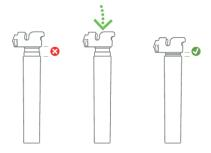
7.2. Tilt the columns and place them correctly on the beam using the guiding notches.
