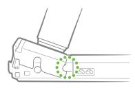
7.3. Fix the column to the beam by pressing down until a "click" is heard and **both** pawls lock the column in the correct position.
