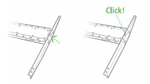
4.3. Mount the cantilever in the other end of the beam.
