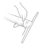
8.2. Fasten the desk panel to the tabletop using the mounting screws.8.3. Fasten the cable to the tabletop using two screws and two cable clamps.
