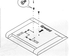
Hook the monitor onto the VESA mount. Tightly Install screws into the bottom two holes, then tighten the top two screws.
