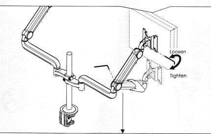
Use the 4mm Allen key provided to adjust the tension to correspond to the weight of the monitor. Twist the Allen key in a clockwise direction for lighter monitors; counterclockwise for heavier monitors.
